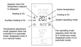
The controller normally displays the measured indoor temperature. To view the setpoint, press one of the ▲▼ buttons. The setpoint will be displayed along with the ◆ symbol for the next 5 seconds.
